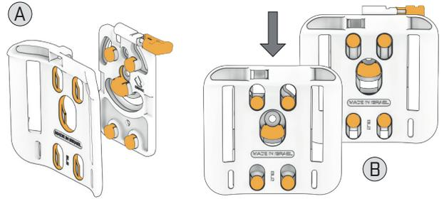
4. Push the latch back in place to lock the insert into the receiver.
