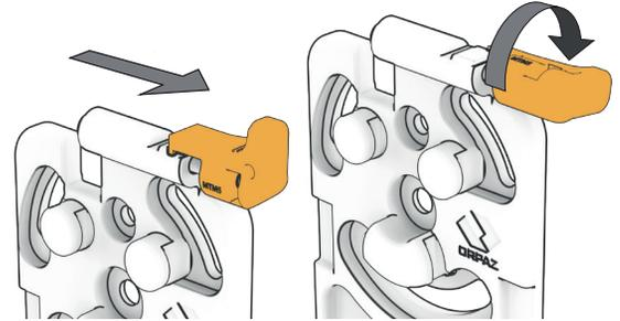
2. Align the insert with the receiver's locking holes (A) Slide the insert down until it stops in place.(B)
