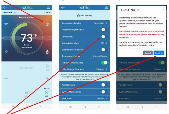
Turn on the Geofencing button and press the Confirm button.
