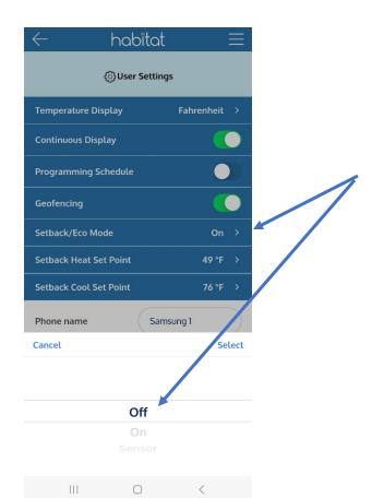
Next, go into the "Setback/Eco" mode setting and change it to off. Press the "Select" icon and then press the "Confirm" button.
