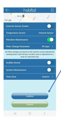
After setting the setpoints for both temperature modes press the 'Confirm' button to store these settings.
