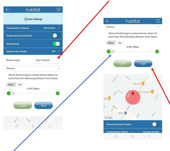
Then, select and adjust the range field to control the unit's activation settings.
