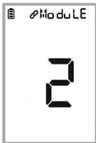
Hold down the **Mode** and **Fan** buttons until a beep is played (3 seconds). After releasing the buttons **MODE** is displayed.
