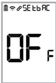
Press **Fan** several times until **SEtBAC** is displayed with either **OFF**, **ON** or **SE<sub>n</sub>**.
