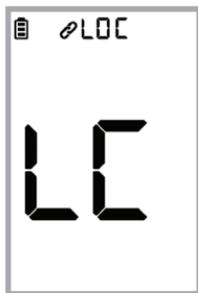
If any button is pressed after locking the keypad, **LC** will be displayed, indicating the keypad is locked. No changes are permitted to Mode, Fan Speed or Set Point while the keypad is locked.
