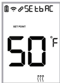
Use the ▲ and ▼ buttons to set the HEAT Set Point. Press Fan to select.
