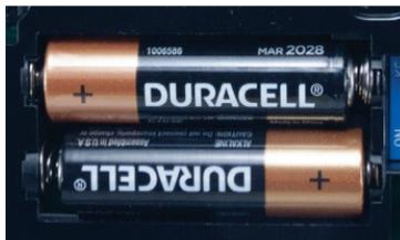
Please insert 2 AA Alkaline batteries (included.) High performance lithium batteries may be used and are recommended on commercial applications.
