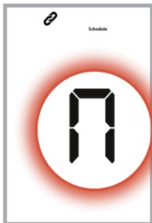
Press **Mode** to scroll back to the Schedule Parameter and use the
