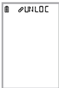
**UNLOC** is displayed, indicating the keypad has been unlocked. The Thermostat then returns to the home screen.
