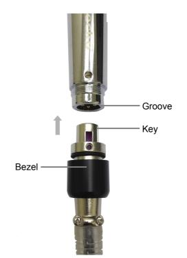
Insert the provided microphone cable with GECKO® Secured Connection <sup>™</sup> XLR (female) connector end into the microphone as shown above. If necessary, rotate the connector to align the key on the connector and the groove in the microphone. Push the connector into the microphone and secure the connection by turning the bezel clockwise until it is tight.
