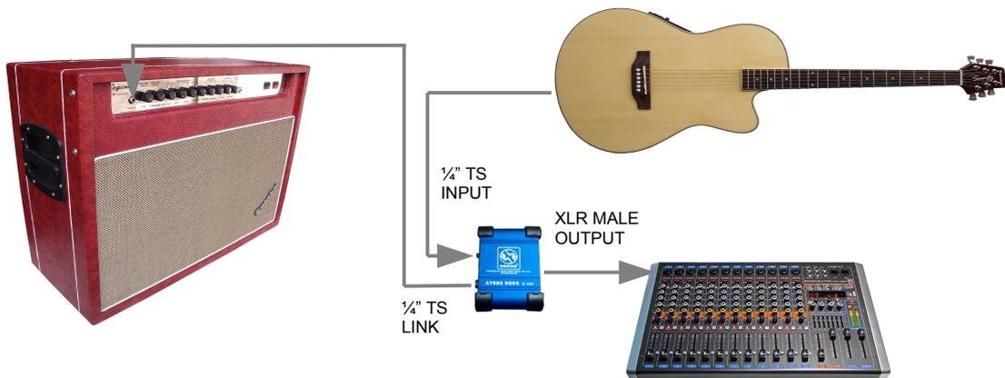
Typical DI Box Setup Diagram
