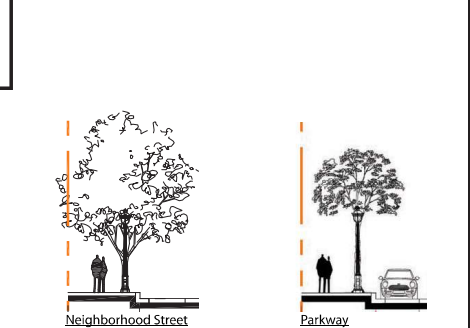
Typical Improvements to Existing Streets: See Section 2.5.1 and Section 3.1.1 for configuration details and construction responsibility
