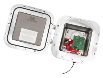
Figure 2. MicroNIR PAT-Lx barrier box interior. Ethernet, power, and trigger connect at the main circuit board through three dedicated ports, using HazLoc-rated connections.
