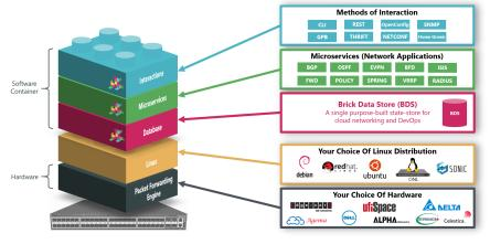
The RtBrick PE Router is delivered as a Linux container and packaged for bare-metal switches within an Open Network Linux (ONL) installation for a seamless experience out-of-the-box. ONL handles peripherals such as LEDs, temperature sensors, and other platform management tasks. The entire networking stack, including the forwarding elements, is implemented in userspace as containerized processes.
