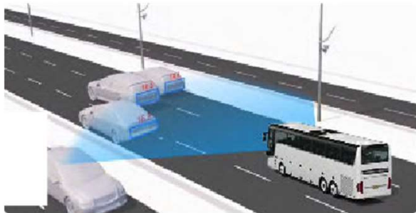
Control de la distancia. (HMW, Headway Monitoring Warning)
