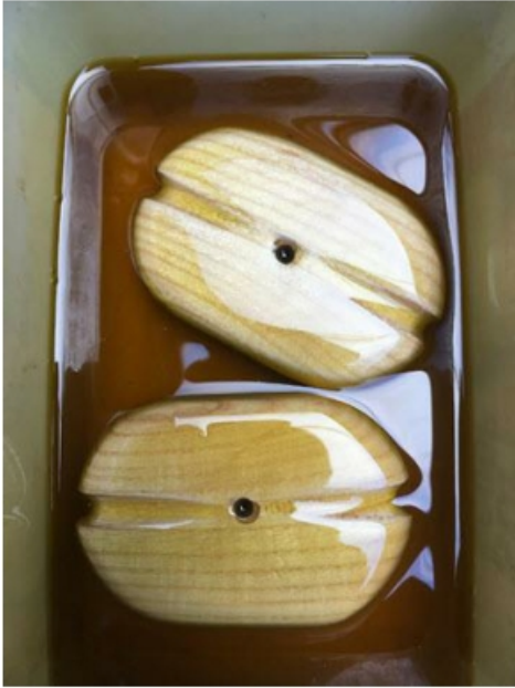
Finished shells soaking in linseed oil.
