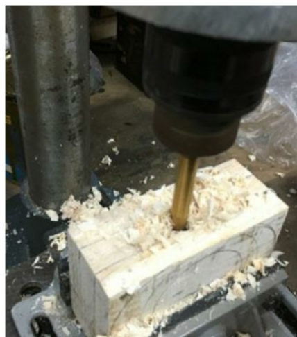
Morticing the shell on the pillar drill.
