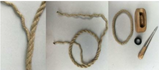
Creating a strop. L-R removing one strand from the rope, laying up the grommet, the finished article.
