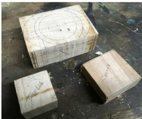
Wooden blanks marked up for block, sheaves and thimbles.
