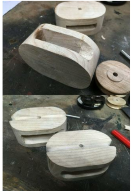
Morticed shells cut to shape.
