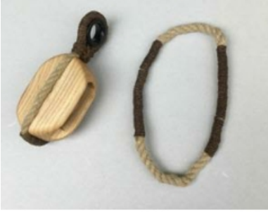
One block with strop fitted and second strop served over to prevent chafe.
