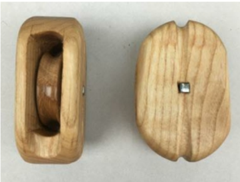
Finished blocks with sheaves in place.
