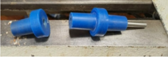
Above: The two simple components of the pen press. One for the headstock spindle and one for the tailstock. Right: The pen press being used in the lathe.
