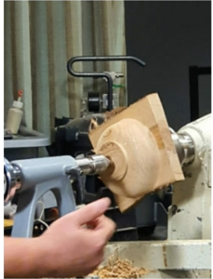
Top Left: Turning the square edged bowl and taking care to keep hands and fingers clear of the wings. Top Right: The underside of the bowl is taking shape.
