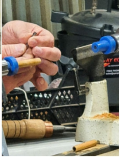
Above: The two simple components of the pen press. One for the headstock spindle and one for the tailstock. Right: The pen press being used in the lathe.
