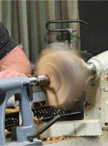
Top Left: Turning the square edged bowl and taking care to keep hands and fingers clear of the wings. Top Right: The underside of the bowl is taking shape.
