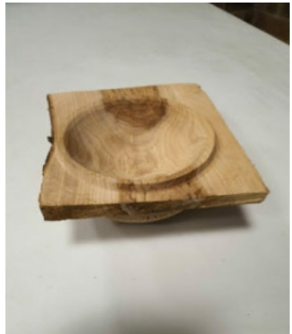
The bowl completed except for sanding and finishing.
