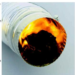
exhaust air. Restrictions should be noted in the inspector's report. Airflow restrictions are a potential fire hazard.
