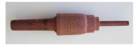
19. Switch from the metal chuck to the new jam chuck for the final work.
