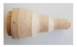
11. Insert the base in the jam chuck and finish the profile
