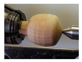
18. Prepare another jam chuck like the one show below. Use the special jam chuck to finish the top. Use a hardwood to ensure a good quality jam chuck. Number 2 morse taper on one end and 5/8" stem for the top to slide on and off.
