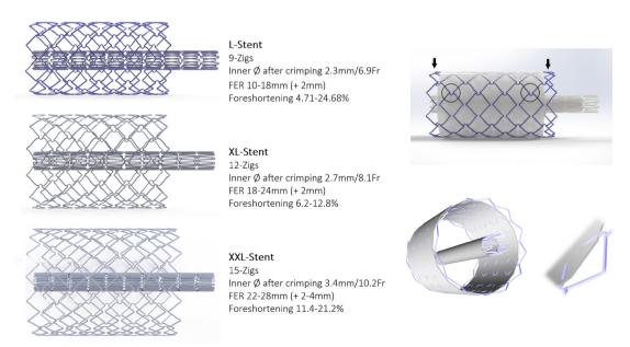
**Figure 1** On the right side, three available sizes of Optimus stents in bare-metal versions: L/9-ZIG, XL/12-ZIG and XXL/15-ZIG. On the left side, Optimus-CVS with end-free sandwich e-PTFE covering design. Note one-half of a row of cells remaining bare segments at either end of the stent (black arrows), and the metal struts sandwiched with inner and outer layers of Nano-ePTFE layers. Note the special hybrid cell design with omega-flex connectors (black circles). PTFE, polytetrafluoroethylene.
