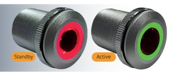
The CTL-SW is a touchless infrared proximity switch, which sits inside a Ø22mm natural anodised aluminium shell. Easily activated without contact, this proximity sensor has a detection distance range from 0 to 10cm. The CTL-SW has an on board LED showing red when in standby mode and green when it is active. Active time is a duration of 10 seconds.
