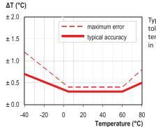
Typical and maximal tolerance for temperature sensor in °C.
