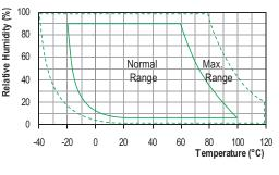
Long term exposure to humidity levels outside of the 'normal' range may temporarily offset **RH** measurements (±3%RH after 60 hours). Once returned to less extreme conditions the device will slowly return towards calibration state
