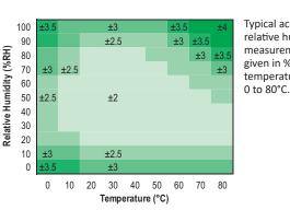
Typical accuracy of relative humidity measurements given in %RH for
