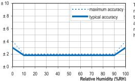
Typical and maximal tolerance at 25°C for relative humidity.
