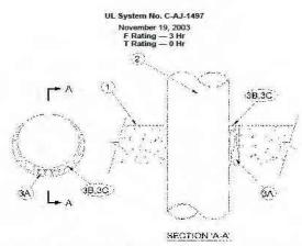
1. Floor or Wall Assembly — Min 4-1/2 in, thick reinforced lightweight or normal weight (100-150 pcf) concrete. Floor may also be constructed of any min 6 in, thick hollow-core Precast Concrete Units\*. Wall may also be constructed of any UL Classified Concrete Blocks\*. Max diam of opening is 1-1/8 in. larger than diam of through-penetrant (Item 2). Max diam of opening in floors constructed of hollow-core precast concrete units is 7 in.
