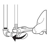
Disconnect the cold water hose from the line. Make sure it is the cold water hose and not hot because hot water will cause the unit to malfunction.
