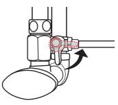
6 Connect hoses to the water inlet and acidic water outlet then open the cold water supply valve.
