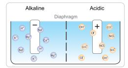
During electrolysis, the cathode has a negative charge and produces alkaline ionized water (pH range 7.5~10) with negatively charged hydroxyl ions, and attracts alkaline minerals - such as calcium, potassium, magnesium, and sodium.
