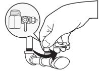
Connect the cold water line adapter to the cold water supply valve as shown.
